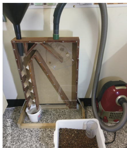
GBDBG's home built, vacuum powered zig zag aspirator.
