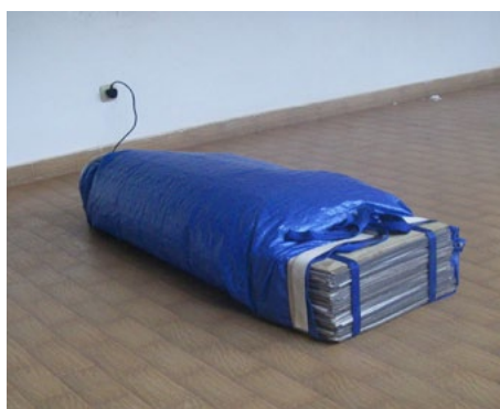
Above: The preferred method of drying herbarium specimens, using an electric fan heater
