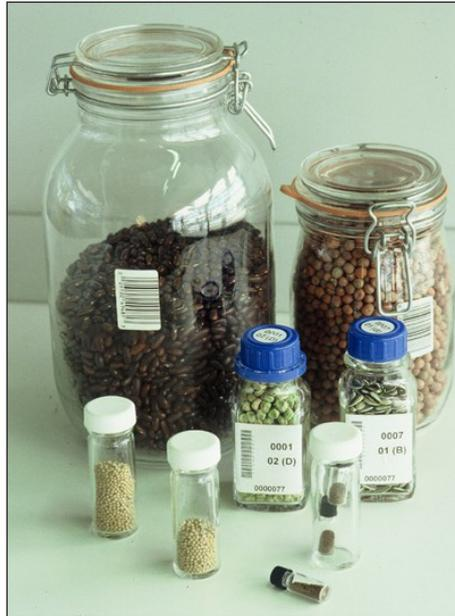
Above: Five types of glass container used at MSB - 3000cm<sup>3</sup> storage jar, 1000cm<sup>3</sup> storage jar, 100cm<sup>3</sup> square bottle, 30cm<sup>3</sup> universal bottle and 2cm<sup>3</sup> vial
