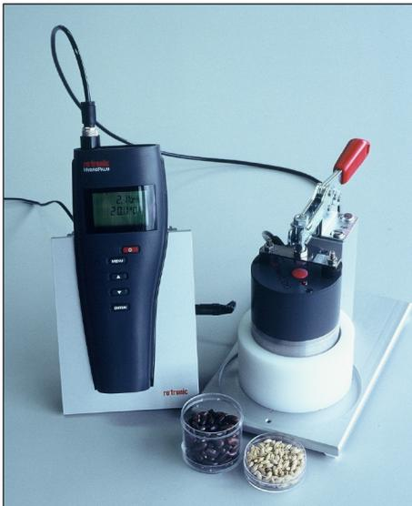
Above: Lab-based Rotronic hygrometer workstation
