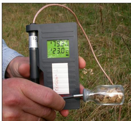
For research applications, it may be necessary to warm or cool the sensor and chamber to the temperature of the seed sample before starting the measurement.
