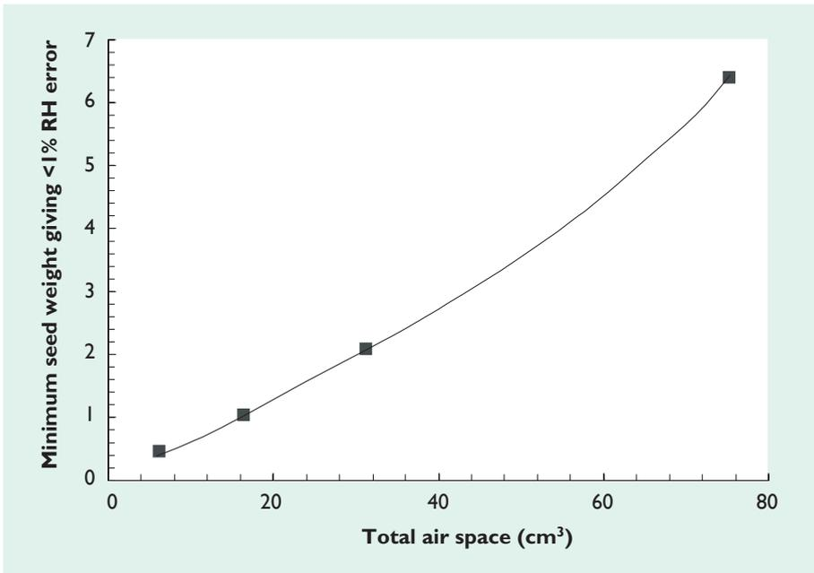
**Figure 20.2** The relationship between the minimum seed sample weight giving <1% RH error in the eRH measurement, and total air space within the hygrometer sample chamber and sensor head, when moist (~80% eRH) *Ranunculus sceleratus* seeds were tested using a Rotronic WA-40 measuring station.
