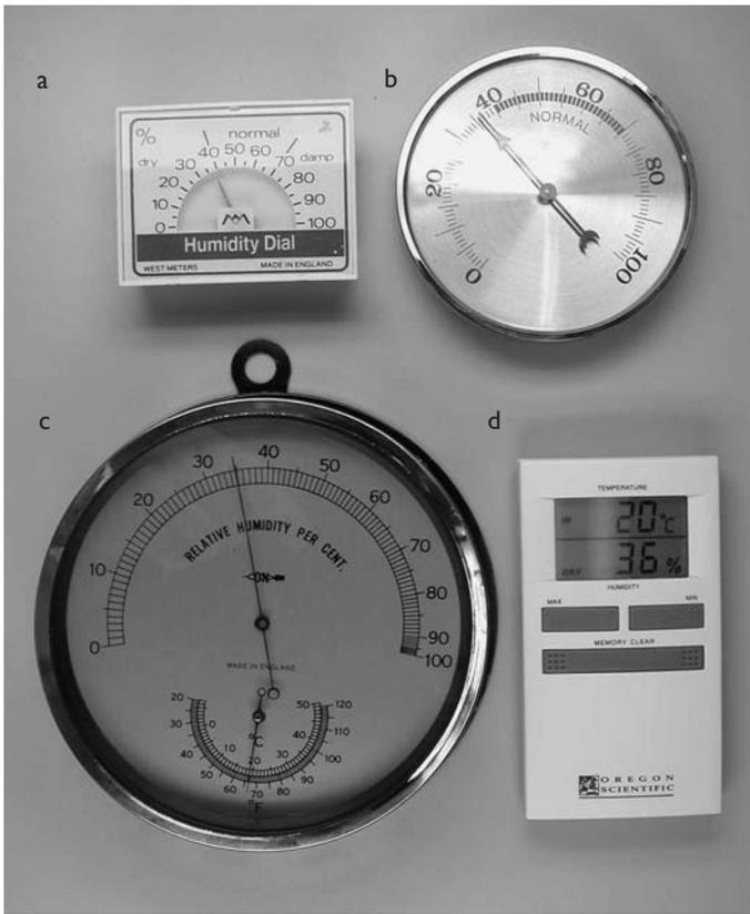
**Figure 20.7** A selection of low-cost hygrometers. a. West Meters humidity dial; b. Pocket Hygrometer (Fisher Scientific); c. Hair Hygrometer (Fisher Scientific) (all mechanical). d. Oregon Scientific Thermo Hygrometer (electronic).
