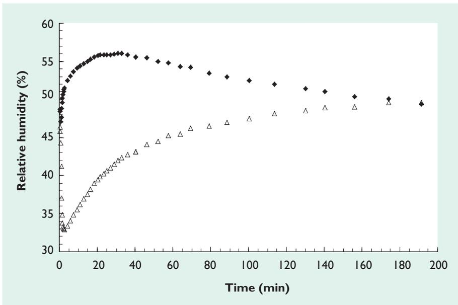
**Figure 20.3** Equilibrium relative humidity measurement of non-equilibrated seed samples. Wheat seeds previously equilibrated to 46% eRH were divided and placed for 24 h at 80% (◆) and 10% (△) RH prior to measurement using a Rotronic AWVC-DIO.
