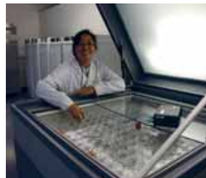
Natali Ramírez Bullón (Universidad Nacional Agraria La Molina, Peru), using a thermogradient plate to study seed germination at 14 different temperatures simultaneously at the MSB. PHOTOGRAPH BY N. RAMÍREZ BULLÓN
