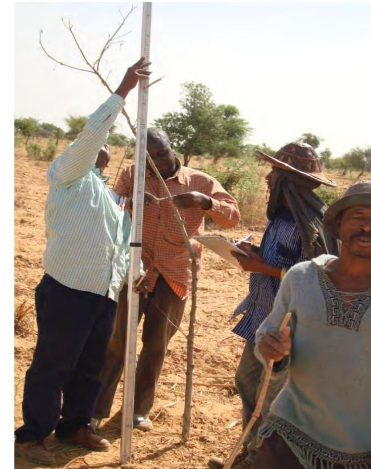
**Photo 6b: Measurement of total height**
