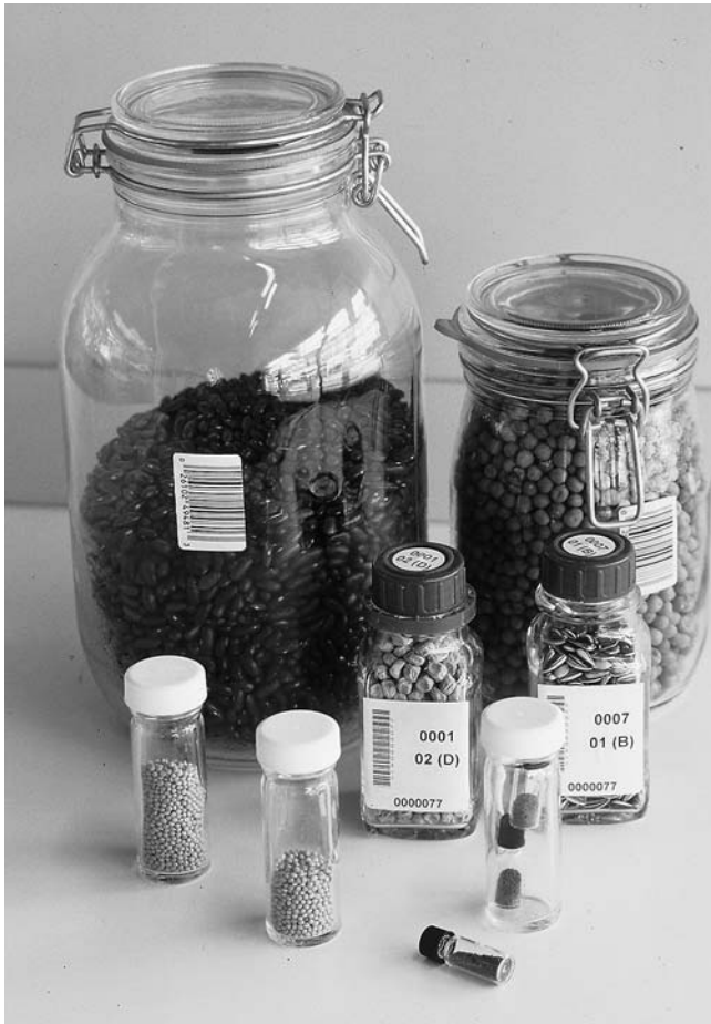
Figure 34.4 The five selected types of glass container currently in use at the Millennium Seed Bank. From rear to front: 3,000 cm 3 storage jar (O), 500 cm 3 storage jar (Q), 100 cm 3 square Schott bottle (E), 30 ml universal bottle (P) and 2 cm 3 vial (K).
