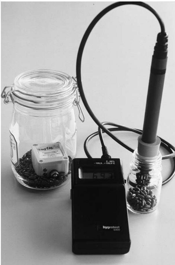
Figure 20.6 Miniature datalogger (Gemini Tinytag Plus) inserted inside jar of seeds (left). Handheld probe-type hygrometer (Testo Hygrotest 6400, no longer available) adapted for insertion into seed container to measure eRH.
